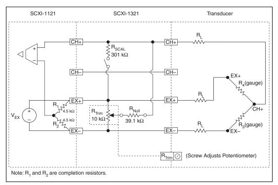
Figure 4. Half-Bridge Nulling Circuit
